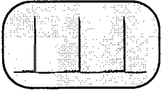
⑭ 31.6 Vp-p IC451 PIN 8
